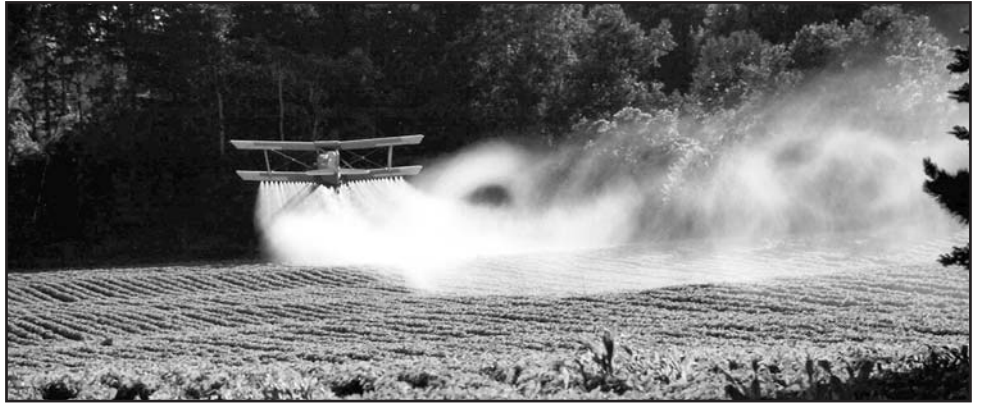
NYS Snap Beans being sprayed with Growers at 3 gal/ac at first blossom on a calm evening at the end of July, 2010. At maturity the canning company estimated them to be 5 tons per acre beans. Photographer was Ted Genagon, retired Kodak company electrician, who helps Bruce Naas part time, and the pilot is Ed Steuber from Albion, NY.
