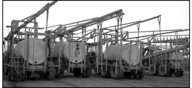
The Valle del Sur sprayers. The drops have nozzles which help to cover both sides of each trellis. This was designed by the farm for this location.
