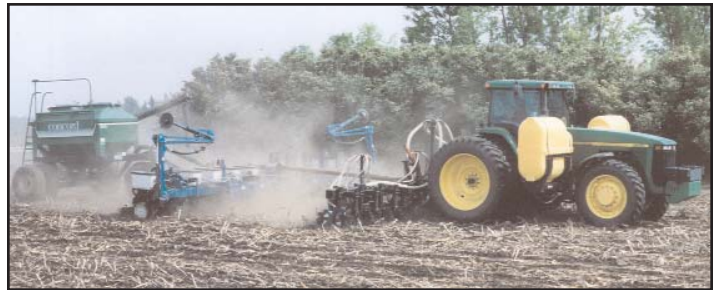
Wiertsema's corn planter pulls a wagon applying 100# hi cal lime in slot ahead of the seed.
